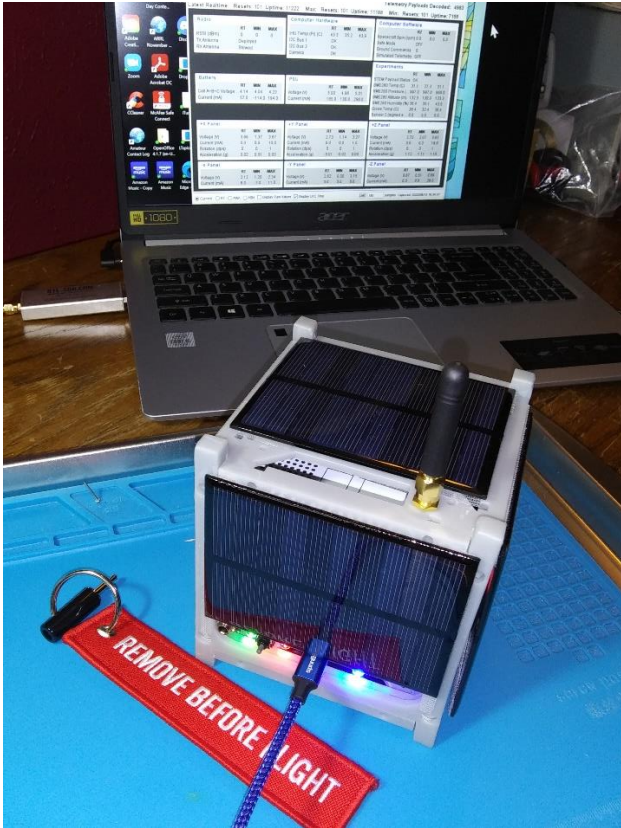
Figure 7: the Cubesat Simulator completed and functioning
